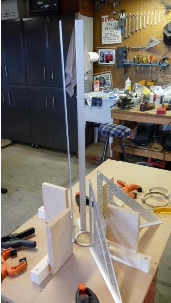
Now fabricate one or two L-brackets from some 1" x 1/8" or 3/16" aluminum bar stock. Make the leg part of the L about 3" long and the length sized to fit the airframes you will be working with. Push the L up against the opposing side of one of the Swanson Squares and secure the leg portion with a couple of screws into the platform. The L will help keep a longer section of airframe more stable in the fixture while you work. Use plumber's pipe band clamps to secure the L(s) to the airframe.
