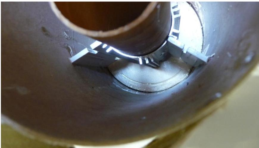
accommodate the larger MMT. Also, the width of the plastic fins furnished with the kit was wider than the two groove sizes provided for on the GROOVE-LOK. Rather than try to shave the sides of the fins down to fit in the grooves and probably lose the squareness needed to align them properly, I offset the GROOVE-LOK radially an appropriate
