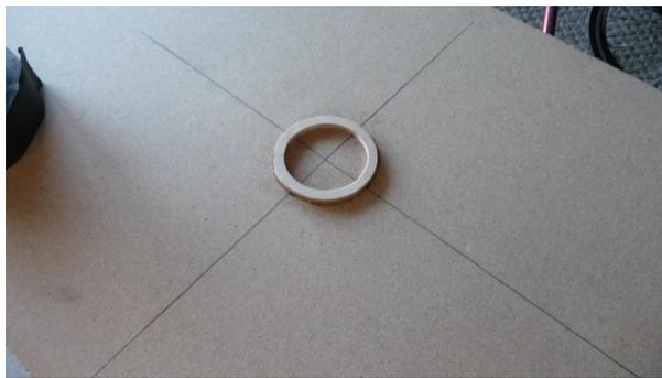
The intersection point of the lines will be the mounting center point for whatever sized centering ring or bulkhead plate you use for your particular project. I was focused on this particular project application and glued a spare 94mm-75mm MMT centering ring in place. It would be better to keep the fixture more multi-purpose. I suggest inserting a 10-32 or similar threaded-insert into the intersection point so you can screw a properly sized bulkhead plate to the fixture. That plate can then
