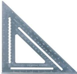
Next, place a section of airframe over the centering ring. Between two of the fins, slide a Swanson's Speed Square (can be purchased at any hardware store for a few dollars) snugly up against the airframe section and drill a couple of holes and secure it in place. 90 degrees around the airframe, secure another speed square in the same manner. These speed squares will assure that the airframe is square relative to the platform.
