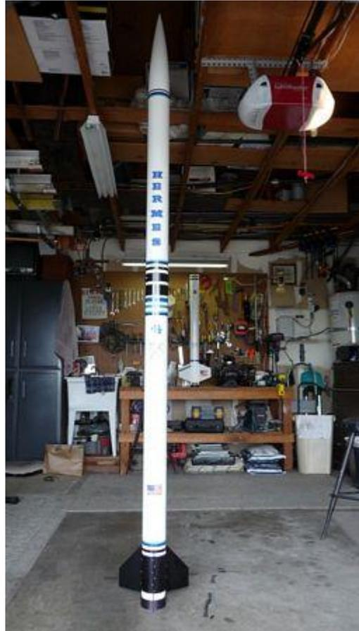
I brought the tube back home and applied some decals and pinstripes in a theme similar to that of Hermes 3 since the payload from that rocket is coupled with the new booster. Back to the paint shop for a final clear coat. I should have had two coats applied since some of the pinstripes peeled away during the initial flight.
